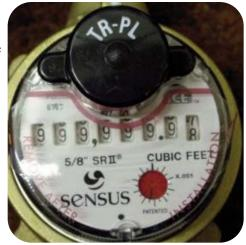
flow indicator, which should not be spinning unless a leak is present. To avoid receiving a surprisingly high water bill caused by an undetected leak, we suggest you check your meter regularly.
