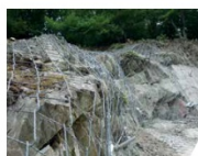
Above: SPIDER® on rock slopes The spiral rope made of three twisted, high-tensile steel wires is characterized by its high puncturing resistance. At the same time it is unobtrusive and can be tightly secured around protruding rock boulders.
