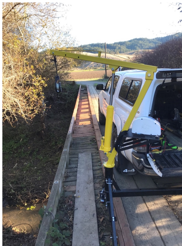
Custom bridge crane used to collect sediment flux measurements.
