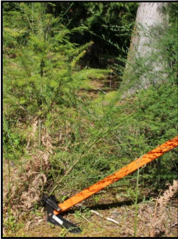
FIGURE 4. STEP 2. The operator's weight – not strength – is used to push the handle to the ground.
