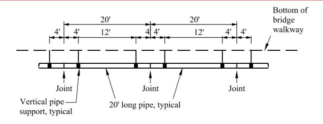
Adjust pipe supports so that they are not directly below railing posts
