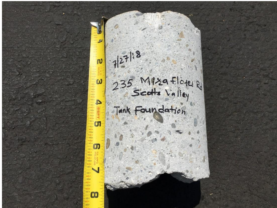
Photograph 7. Core #2 tested for the compressive strength of concrete.
